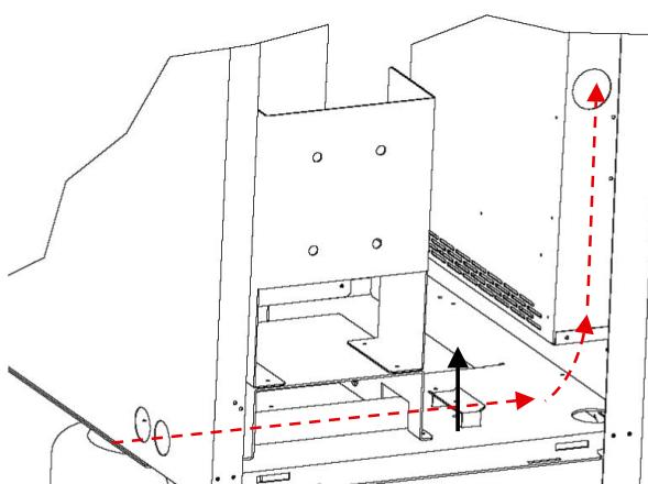
The power cable must be run through the guide tubes, inserted into the side of the control box and secured by means of the strain relief.
