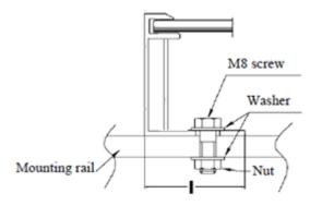
Figure 2: PV module installed with Screw fitting method
