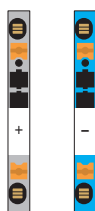
Connection of the PV strings, as well as connection to the inverter
